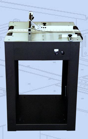
The 240BT Bump Turn provides an inline solution for rotating products 90 degrees from their infeed orientation. This unit is capable of turning a large range of material sizes and thicknesses left or right.
