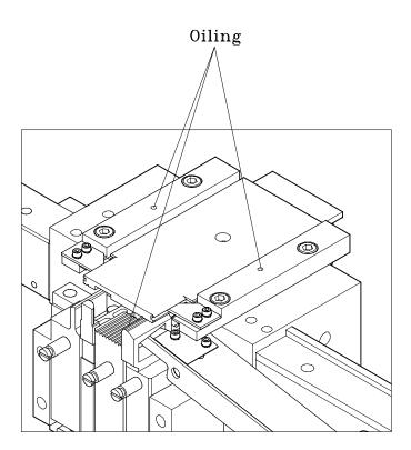
Lubricate the marked points weekly. Only use resin-free branded oil for lubrication. All other assemblies are maintenance-free. Remember that the strap guides and the sealing unit have to be kept clean!
