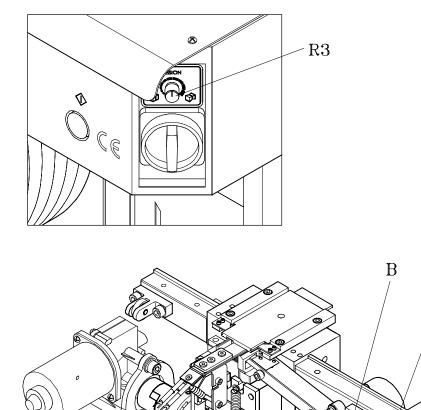
If R3 (strap tension adjustment) is on MAX position make sure that A is turned clockwise until the strap is no longer sliding between rollers B and C. Reverse action to reduce strap tension.
