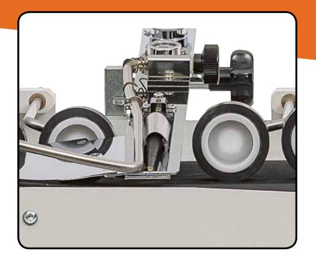
These envelope sealing machines have a large water reservoir with visible water level, automatic level control and a self-cleaning moistening roller. The moistening intensity is adjustable. A continuous adjustment of the belt speed enables individually selectable output of up to 18,000 letters per hour.
