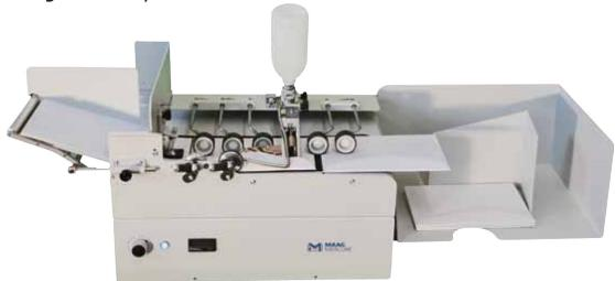
These modern envelope sealing machines seals all common envelope formats from C6/5 up to C4 pocket cleanly and quickly.
