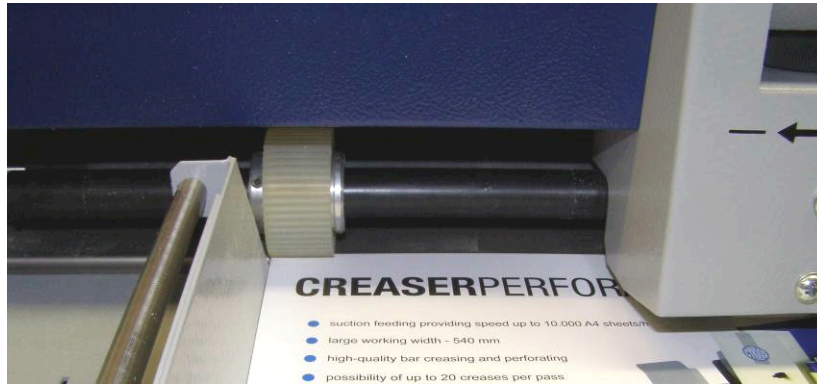
Fig. 12: Correct adjustment of the feeding wheels
