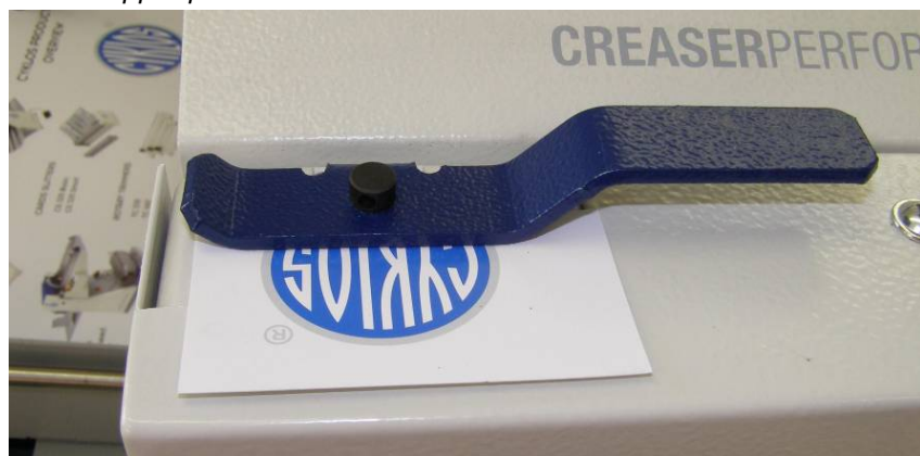
Fig. 18: Defining the gap of the friction feed system by placing paper under the callipers
