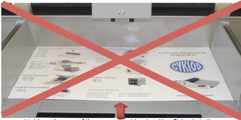
Fig. 8: Incorrectly prepared table – absence of the magnetic strips (position 5) leads to the paper deformation.
