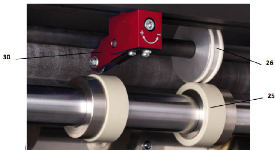
Fig. 11: Setting Rotary Perforating and Cutting
