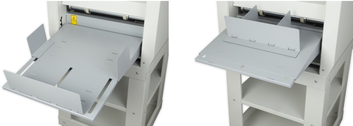
Fig. 12: Setting Delivery Table
