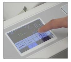
**TOUCH SCREEN** The LED touch screen sets up 36 standard folds automatically at the touch of a button. Up to 24 custom folds can be stored in memory.
