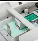
A belt fed, air suction system allows problem-free feeding of coated stock.
